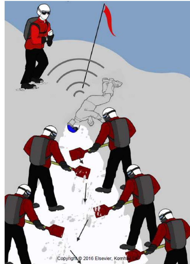
AVALANCHE SAFETY: Manuel Genswein's V-Shaped Snow Conveyor Belt Shoveling Technique
